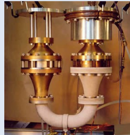
ThermoAcoustic Life Science refrigerator TALSR (1991) Penn, State
