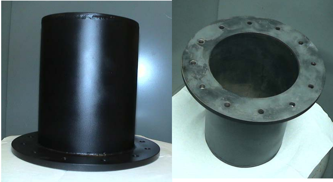
Figure N.8: Main body of the receiver/boiler.
