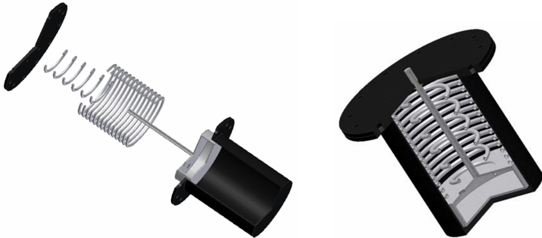
Figure N.6: a) Exploded \frac{3}{4} view of receiver/boiler. b) \frac{3}{4} view of assembled receiver/boiler.
