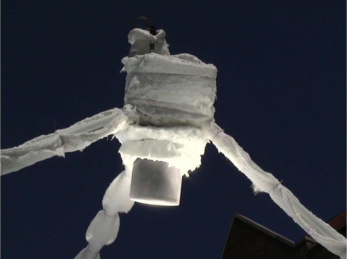
Figure N.12: Receiver/boiler being submitted to concentrated solar insolation.
