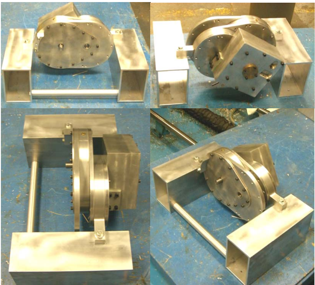
Figure 2.11: Completed assembly of steam turbine and drive train.
