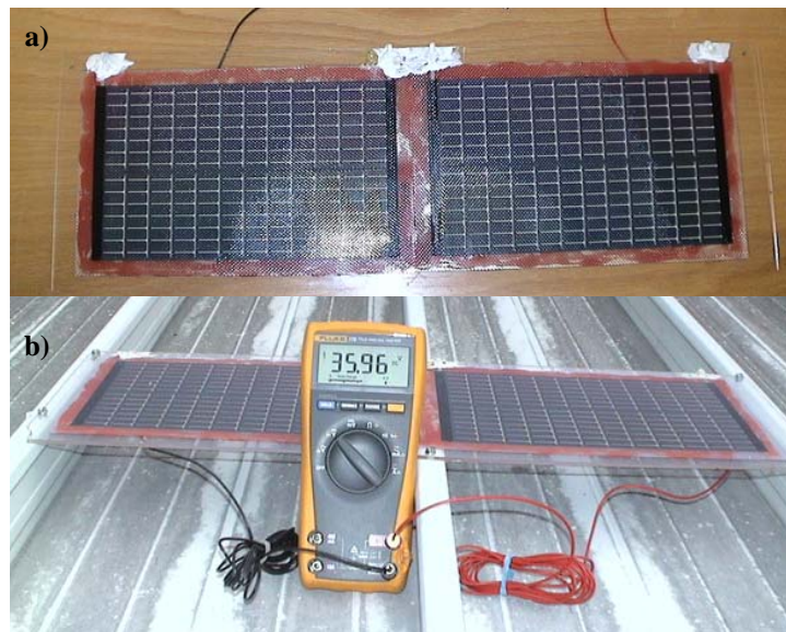
Figure 2.21: a) The thin-film solar panels assembled together in series on plexi-glass sheet. b) The solar panels mounted and producing 35.96 volts under intense sunlight.
