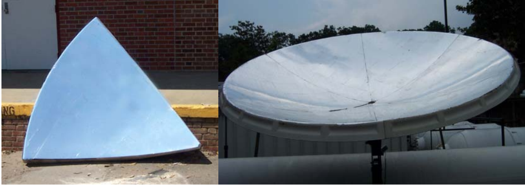
Figure 2.1: a) Pie-shaped section of the dish coated in Aluminized Mylar. b) Assembled dish with surface area of 11.7 m 2 .
