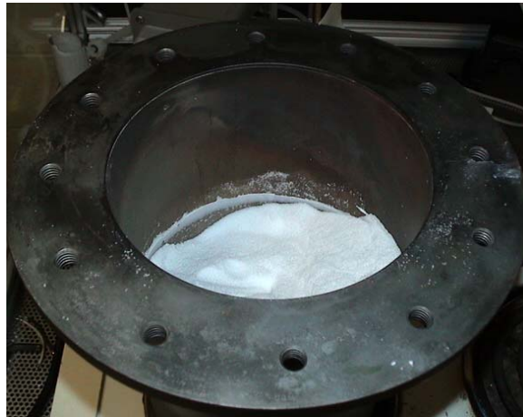
Figure 2.4: The Draw Salt mixture being mixed in the receiver.
