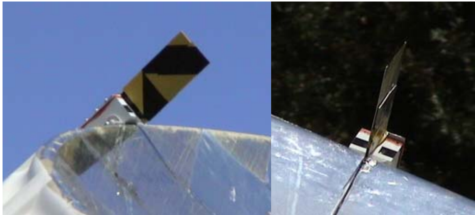
Figure 2.18: Tracker module housing painted white and shading added.
