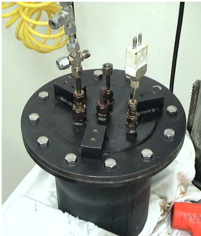
Figure N.10: Receiver/boiler assembled with thermocouple and feed-tubes.
