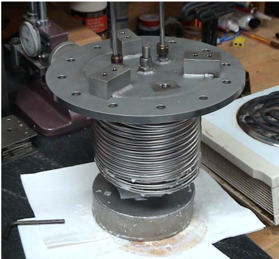
Figure N.7: Image of the actual receiver cap, inner and outer coils, and water drum assembled.
