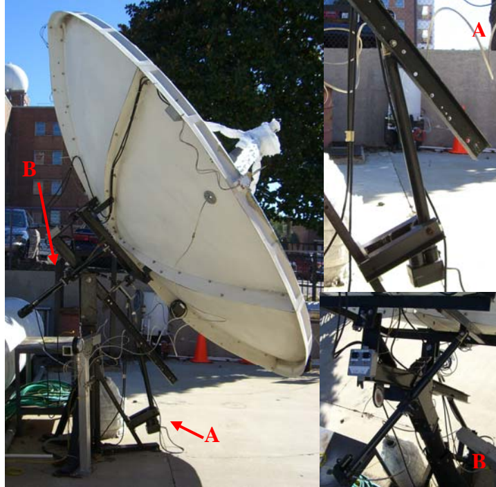
Figure 2.14: Images of the frame with attached actuators. A) Altitude (North/South) control actuator. B) Azimuth (East/West) control actuator.
