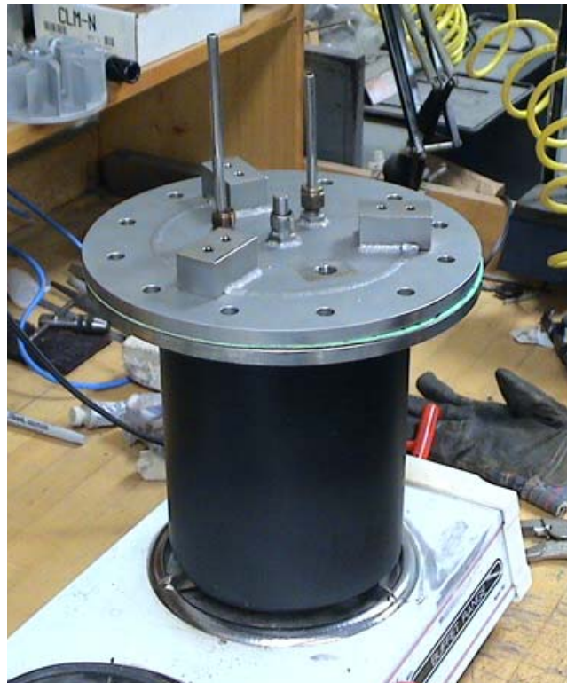
Figure N.9: Assembled receiver/boiler being heated on electric burner for initial mixing of the draw salt thermal bath.
