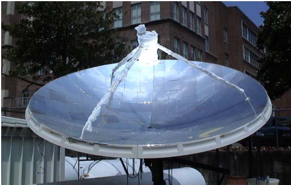
Figure 2.6: Receiver assembled and positioned in focal region of concentrator. Receiver and supporting structure of receiver wrapped in super wool insulation.
