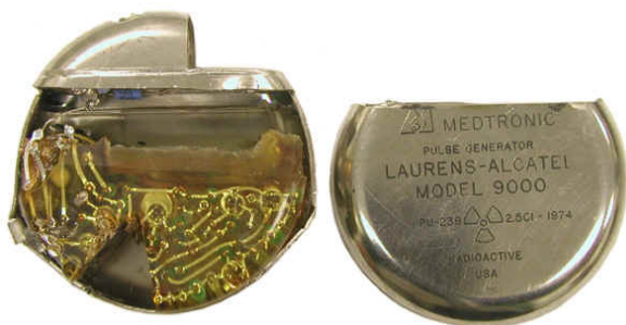
Figure 2.2. A plutonium powered pacemaker. The plutonium has been removed; it fit into the slot on the top left. Hundreds of these were implanted in patients with no ill effects. Cold fusion will also scale down to devices this size or smaller, and it will scale up to any size you like.
