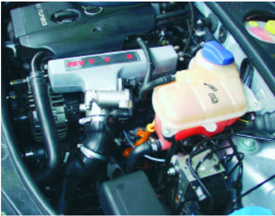
VCR-Engine In-Vehicle Installation
