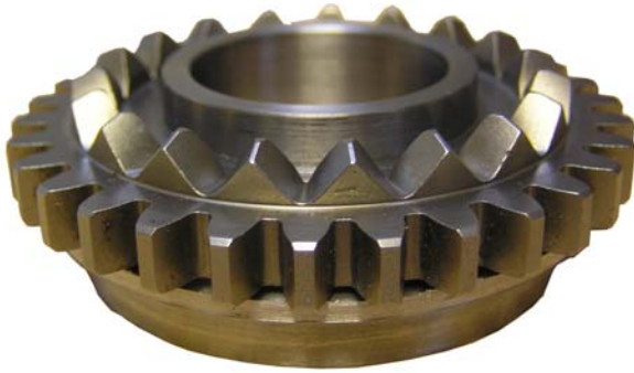
Example (left) of the face gear used in the 125cc RCV engine
