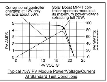
connects the module to the battery and therefore forces the module to operate at 12V. By forcing the 75W module to operate at 12V the conventional controller artificially limits power production to  $\approx$ 53W.
