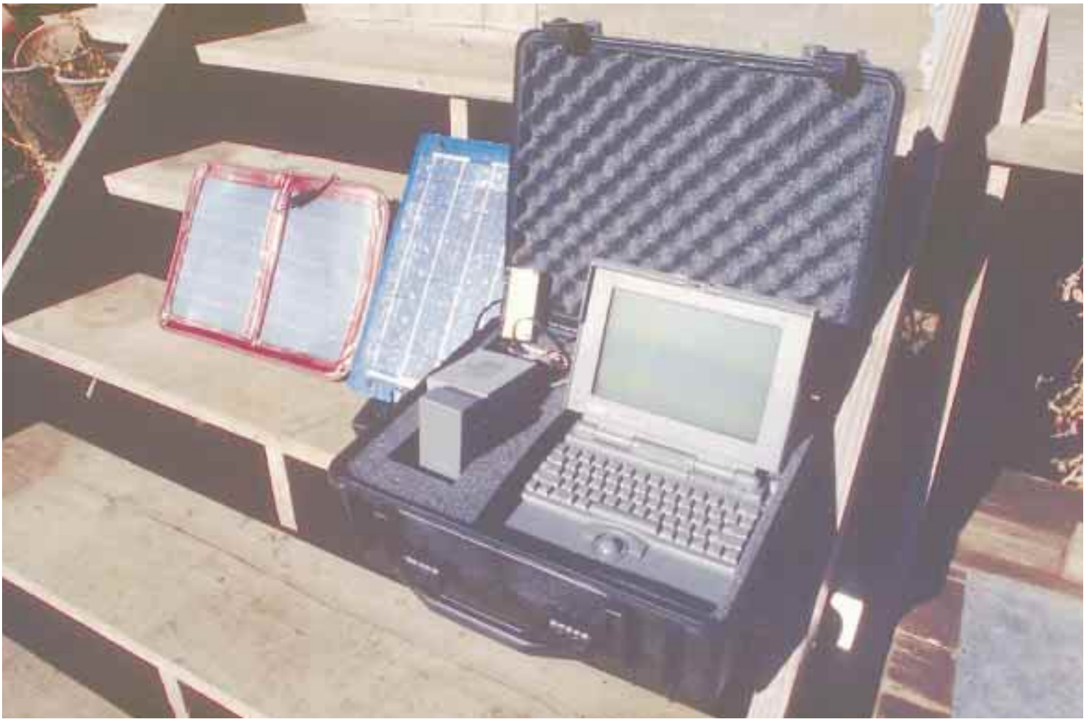
Above: A portable solar-powered system runs computers and communications equipment. The system recharges from the sun, an automobile, or from the electric grid wherever you are. Photo by Richard Perez
