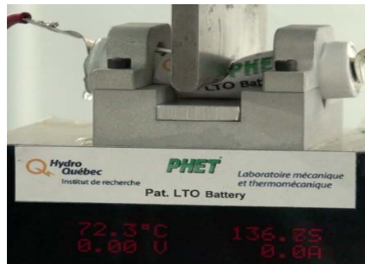
Figure 2. Photograph of a standard 18650 cell after crush test - no smoke and no flames were observed.
