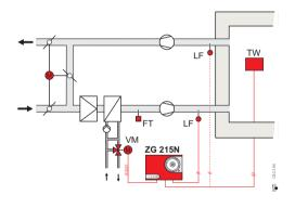
ZG Control Unit VM Servomotor ZR Heating mixing valve LF Air duct sensor
