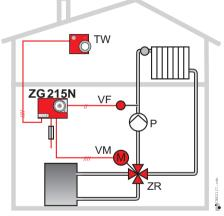
Control Unit ZG VM Servomotor ZR Heating mixing valve
