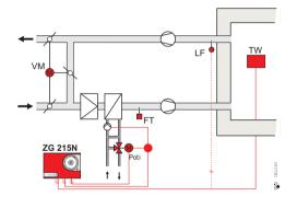
ZG Control UnitVM ServomotorZR Heating mixing valve
