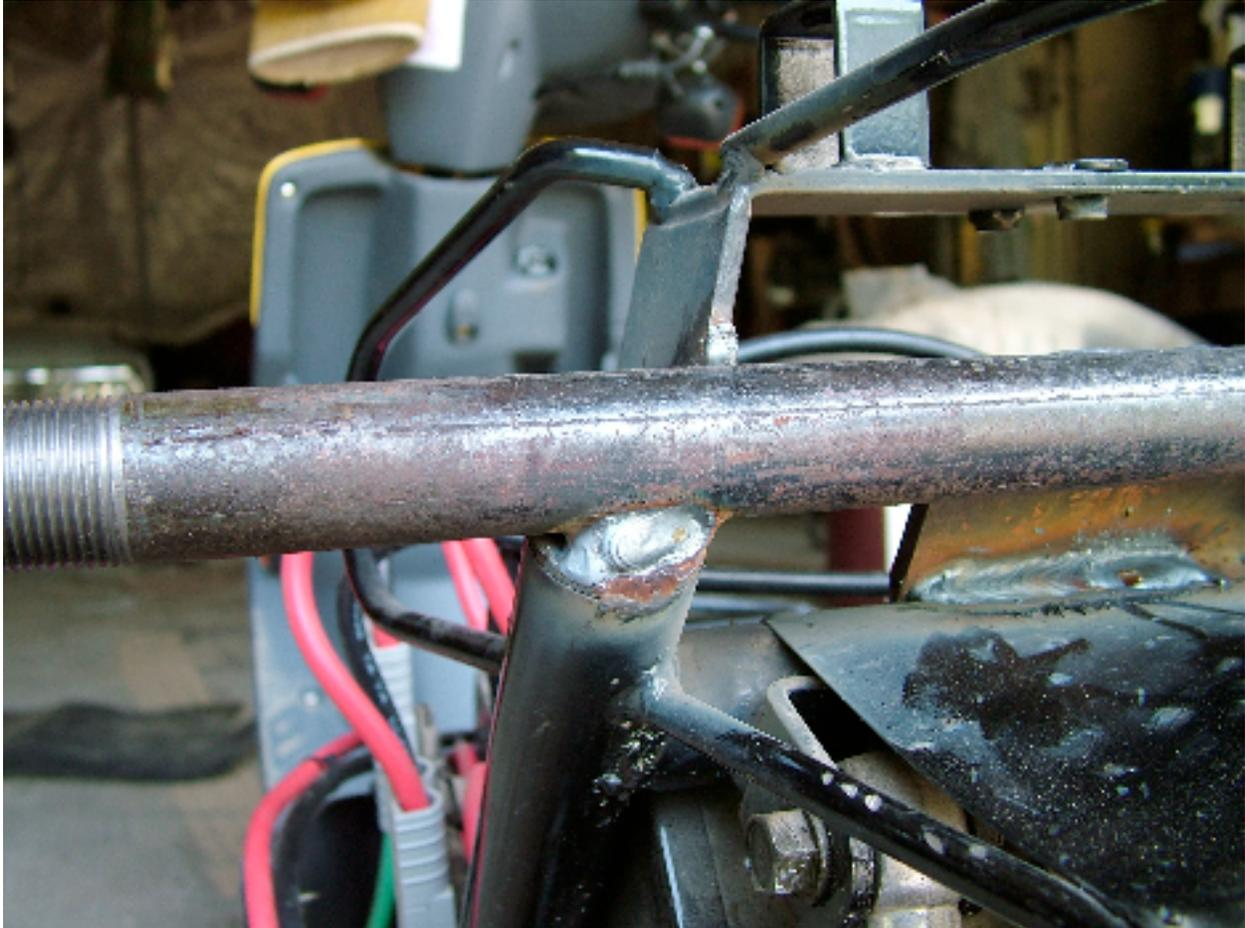
On the end of the vertical bike frame a bed of welding rod material is built up under the main pipe to act as a support so the main pipe for the panels won't flex or bend during travel. The bike was wiped clean after welding, reassembled, and driven home to begin attaching of the panels.
