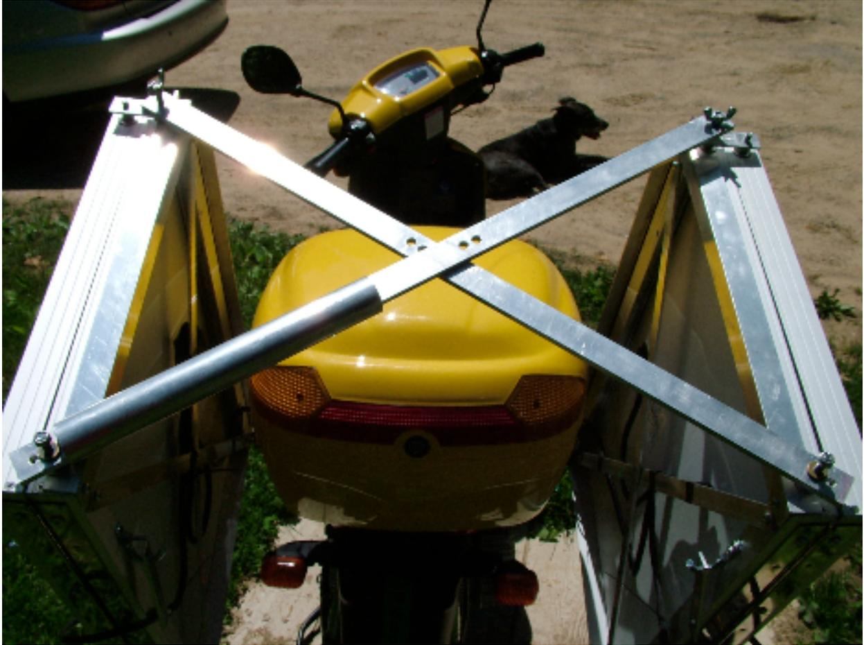
With the panels properly mounted, the next step is to make the crossover/locking mechanism to lock and support the panels in both driving and charging positions. This piece needs to be both strong as well as easy to use. The purpose of the crossover is to create a triangle joint between both sets of panels to keep them from moving while driving down the road.
