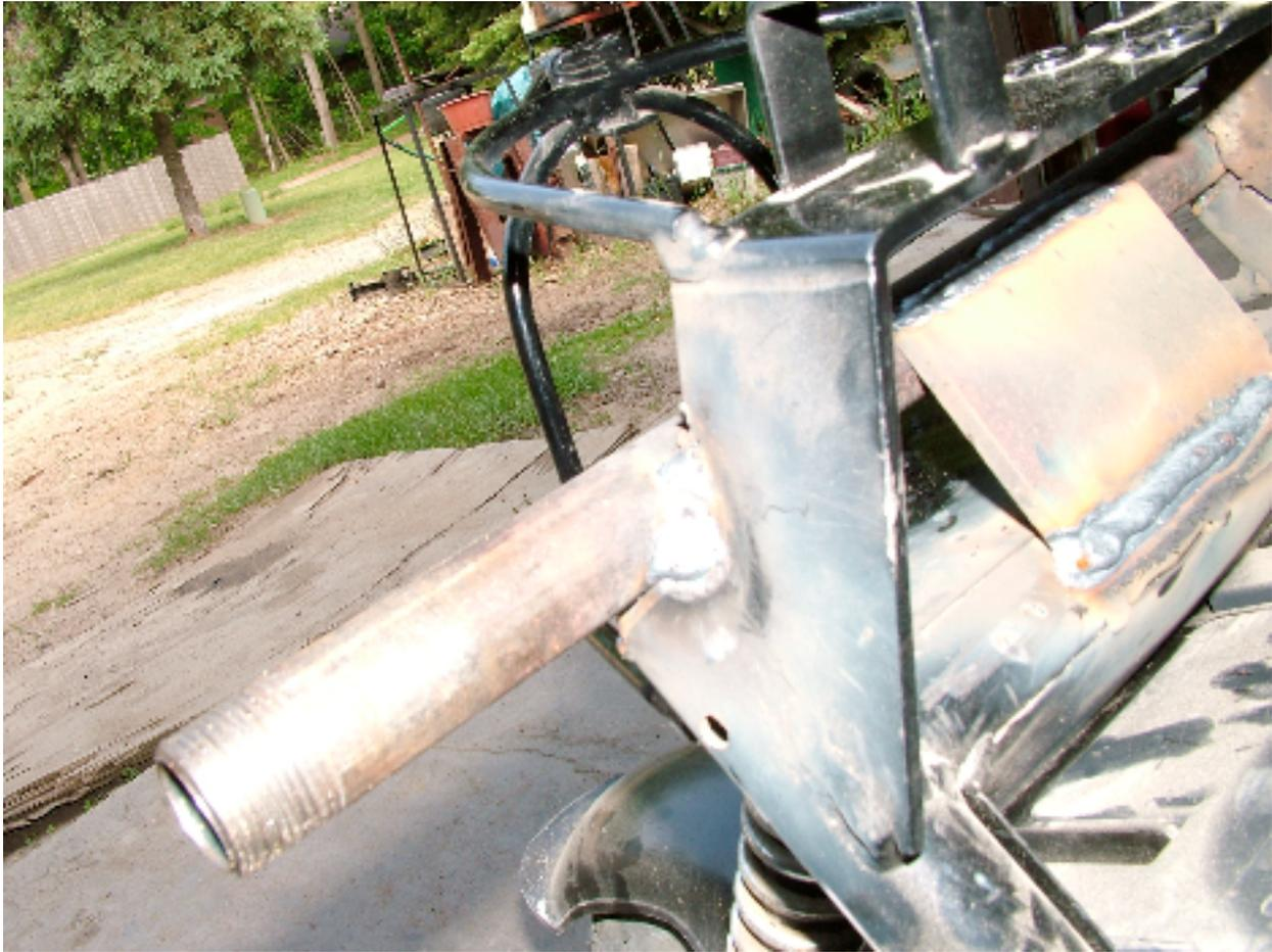
The metal was scrapped clean at the welding points on the bike frame. The main pipe was carefully measured and held in place and then remeasured. The main pipe was tac welded in place, rechecked for alignment, then fully welded. A 2 1/2 inch by 4 inch piece of flat 1/4 inch stock was welded to the bike frame cross bar connecting the top of the bike frame together.
